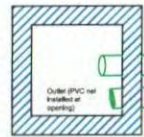
Inspection Pit 600mmX600mm
