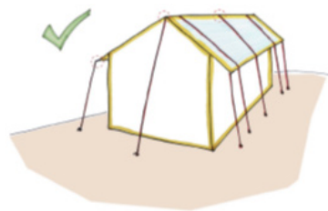
Image 31: Tying the shelter to the metal footing
