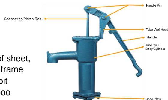
Component of Hand Pump
