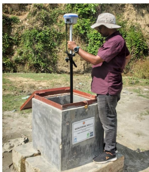
Figure 2.5: Elevation survey of the monitoring well platform.
