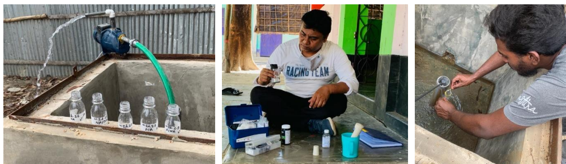
Figure 5.2: Photographs showing (left) sampling for laboratory analysis of water chemistry, (middle) field kit test of arsenic in the field and in-situ field parameter measurements, and (right) sampling for microbiology (hand was sterilized before sampling).
