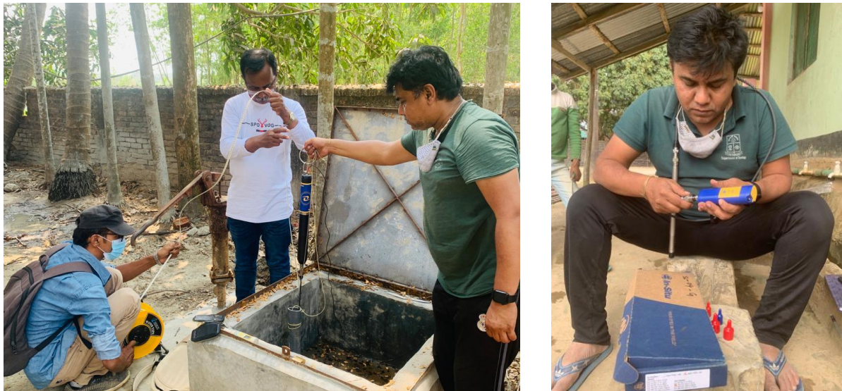
Figure: 4.1: Photographs showing (left) installation of telemetric unit, (right) downloading of data from non-telemetric unit.
