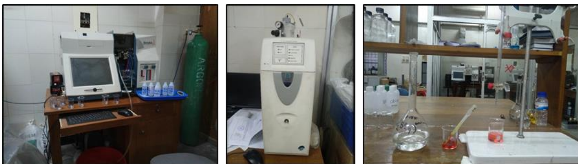
Figure 5.3: Equipment and methods used for the chemical analysis. From left to right - Atomic Absorption Spectrometry (AAS), Ion Chromatography (IC), and Acid based titration
