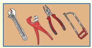
Plumbers and pipefitters use wrenches, pliers and pipe cutters.
