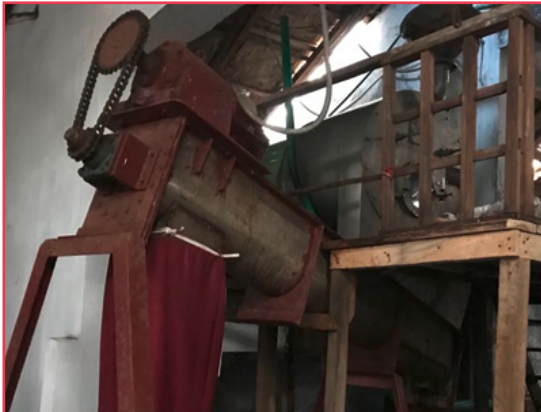
Image of a centrifuge machine in a salt refinery mill. © Khairul Islam.
