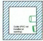
Inspection Pit 600mmX600mm
