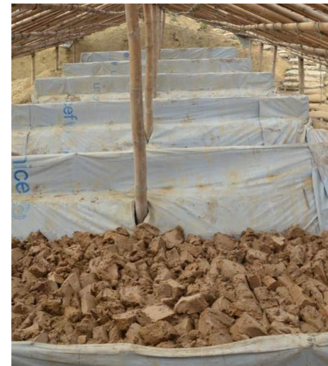
Image 26: Lime 1 - Drying bays
